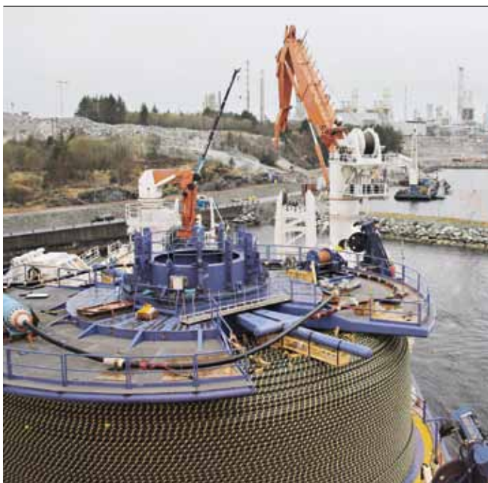
8 The cable-laying vessel in Mongstad, where the cable connects to the shore
